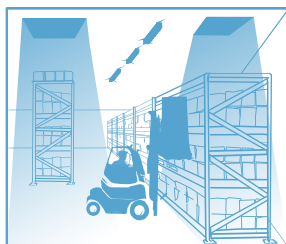
With sufficient ambient lux level, the light keeps off even when motion is detected.
