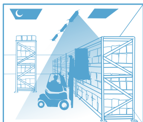
Light is on when the sensor detects the motion and the ambient lux level is insufficient.
