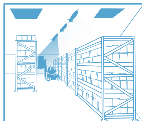
When no more motion is detected, the light dims entering standby mode after hold time.
